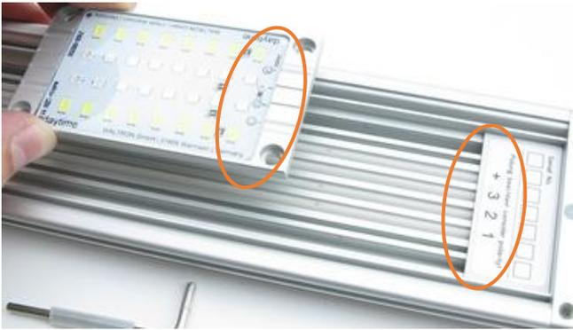
Selecting the module position and inserting (not yet pressing) the module, **respecting the correct polarity:**
