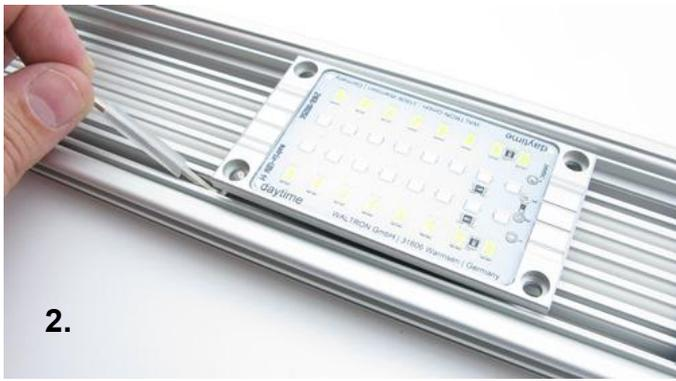
**⚠ Attention! The rubber coating of the short key leg must be present and completely cover the key edges so as not to damage the underside of the module.**
