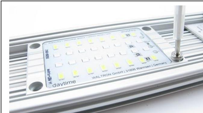
Loosening and removing all screws
