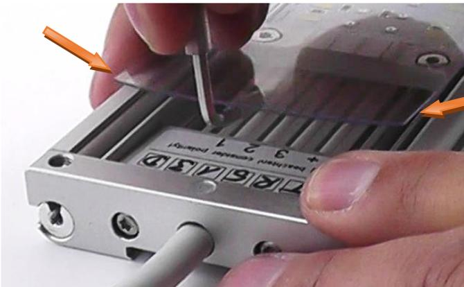
... until the pane edges "jump" out of the profile grooves
