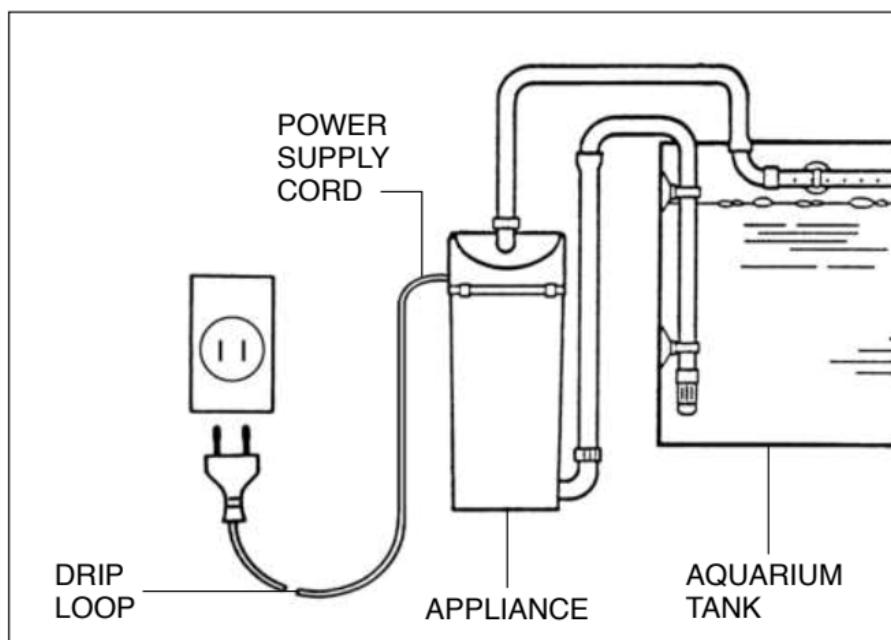
A "drip-loop", shown in the figure, should be arranged by the user for each cord connecting an aquarium appliance to a receptacle.
