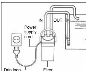
For your own protection, it is advisable to make a loop in the electrical cable to catch drips and prevent any water running along the cable from entering the socket.
