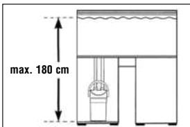
To achieve optimal operational safety there must be a maximum of 180 cm between the surface of the water and the bottom of the filter.
