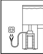
For your own safety, we recommend to form a drip loop with the connection cable to prevent any water running along the cable from intruding into the socket.
