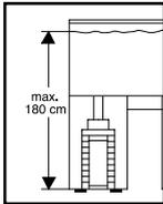
Take the erection height into account when selecting the device's operation site. To assure optimum functional safety, observe a max. clearance of 180 cm between the water surface and the filter bottom.
